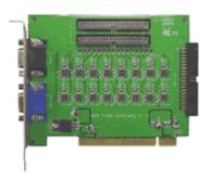
The GV-Loop Through Card is designed to take the video signal directly from the GV Capture Card, without internal device processes, and then split it into 16 signals while maintaining video quality.
